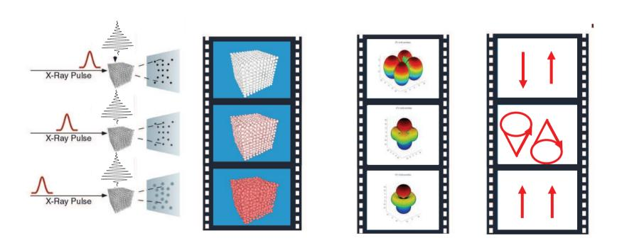
Ultrafast X-rays probe changes in atomic, electronic and magnetic structure following electronic or lattice excitation.
